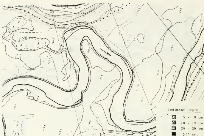
Figure D15 Topographic Map of Sediment Deposition - Zone # 42
