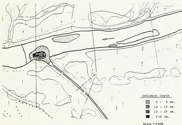
Figure 12 Topographic Map of Sediment Deposition - Zone # 26
