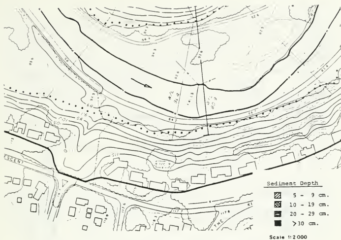
Figure D1 Topographic Map of Sediment Deposition - Zone # 22
