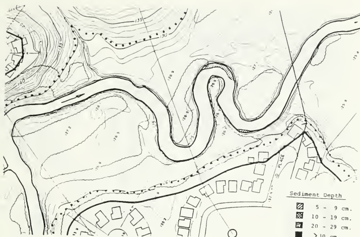
Figure D13 Topographic Map of Sediment Deposition - Zone # 40
