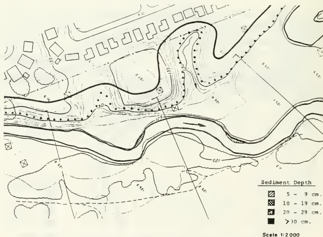
Figure D12 Topographic Map of Sediment Deposition - Zone # 39
