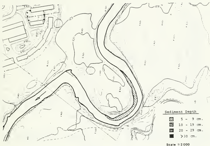
Figure 15 Topographic Map of Sediment Deposition - Zone # 37
